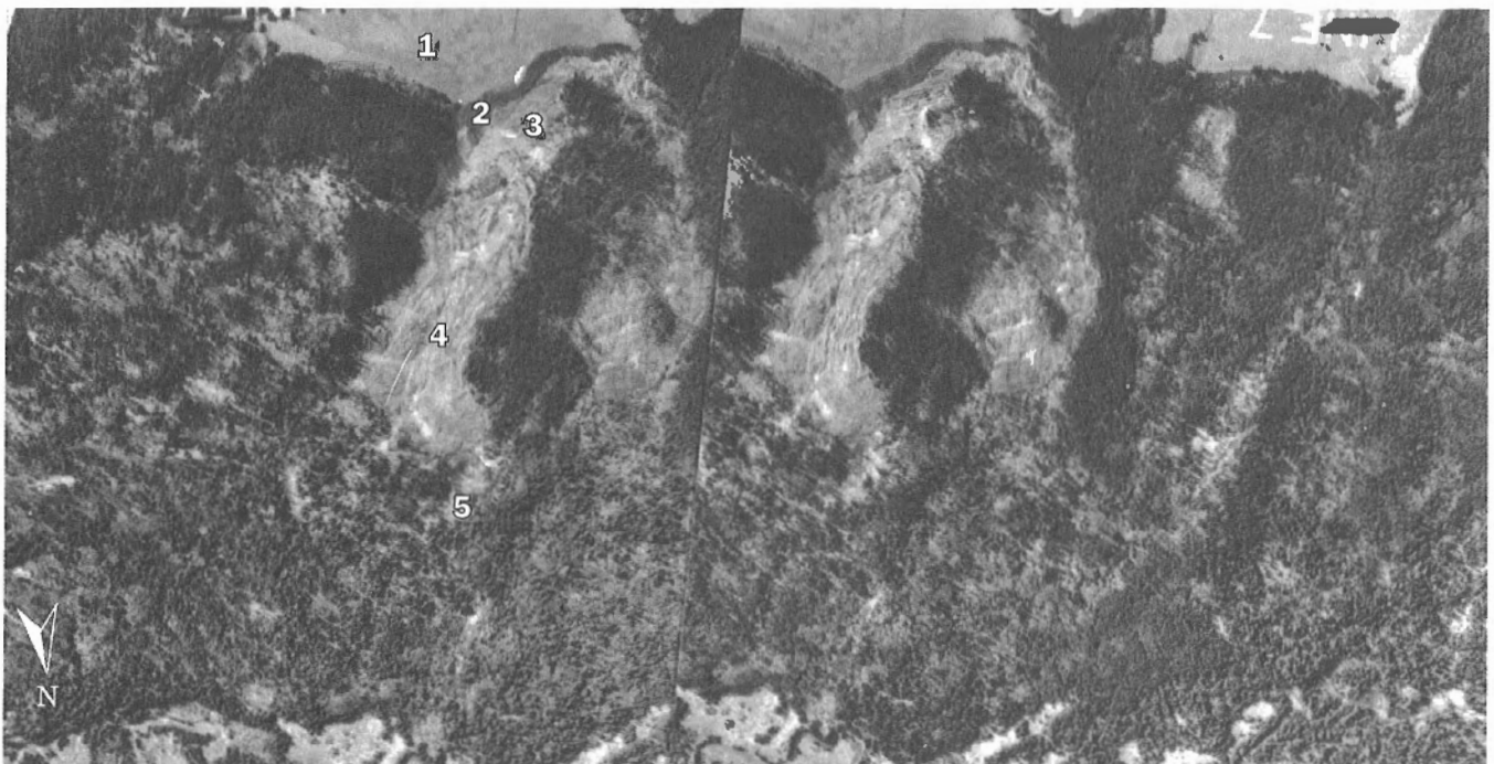
Figure 2. Stereo-pair of Police Point landslide, south side of Battle Creek. 1) upper plateau surface; 2) upper scarp exposing Cypress Hills Formation; 3) rotated slump blocks; 4) gully erosion within Cretaceous sediments; and 5) sediment washed from landslide into the forest. Airphotos AFL W AS2343-249, 250. See Figure 3 for ground photographs.
