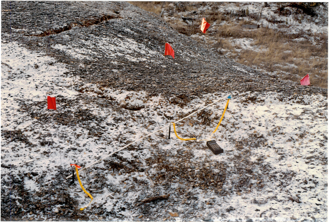
Plate 4. Slope 31A, Unnamed Creek South, KmP 84.5, Oct. 7, 1993. Handheld microprocessor controlled digital thermometer probes are used to measure temperatures in the wood chips to a depth of 30 cm in order to delineate the extent of the hot spot.
