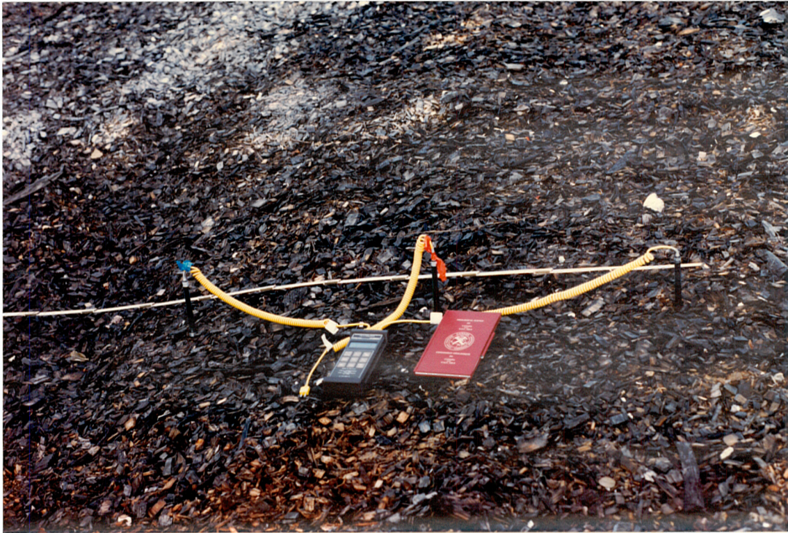
Plate 27. Slope 79, Whitesand North, KmP 279.0, Oct. 3, 1993. Monitoring wood chip temperatures at 30 cm depth with the digital thermometer probe in an attempt to locate the hot spot.
