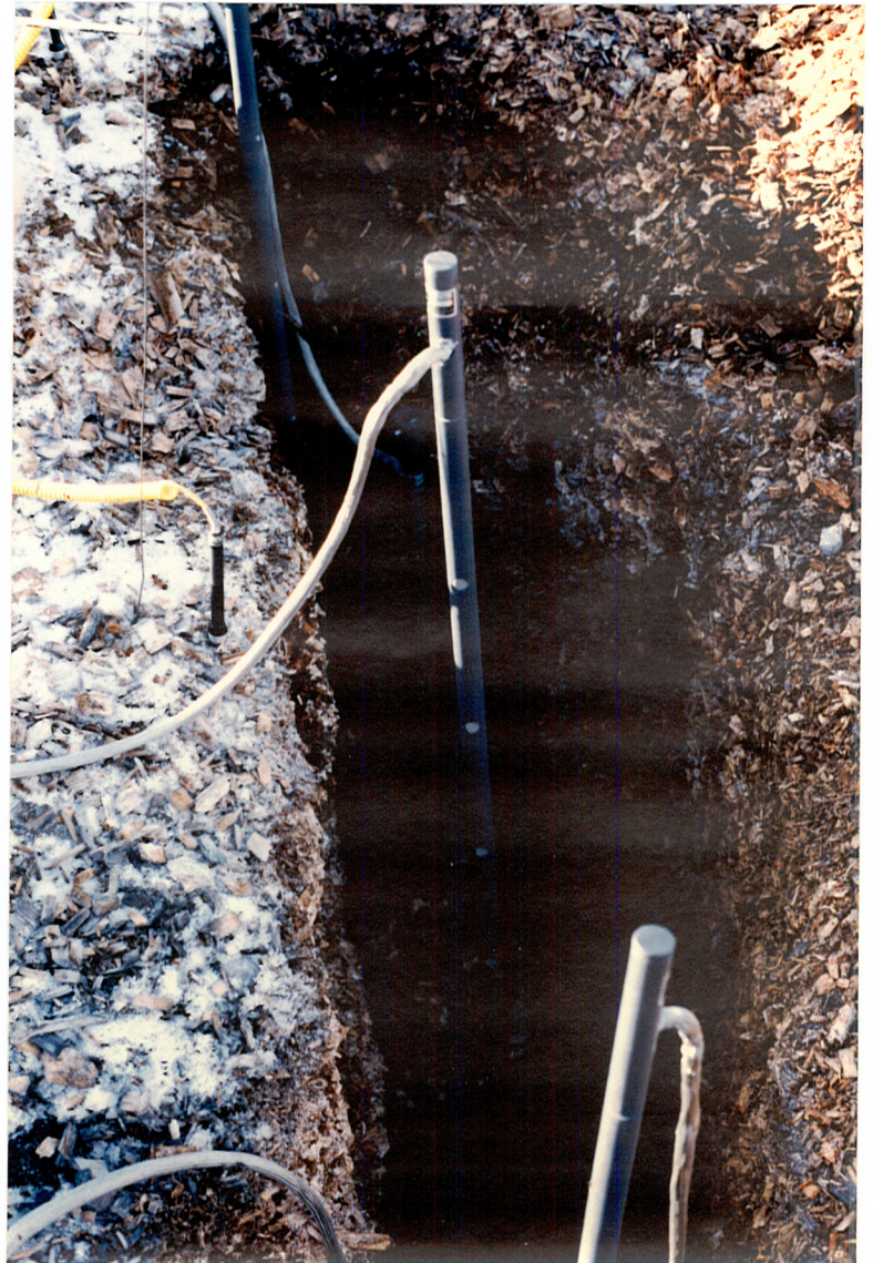
Plate 4. Slope 31A, Unnamed Creek South, KmP 84.5, Oct. 7, 1993. Handheld microprocessor controlled digital thermometer probes are used to measure temperatures in the wood chips to a depth of 30 cm in order to delineate the extent of the hot spot.
