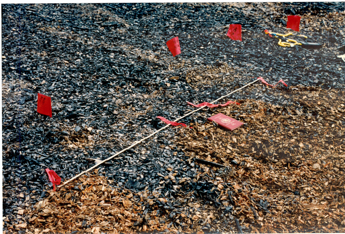
Plate 39. Slope 112, River Between Two Mountains, KmP 352.3, Oct. 6, 1993. Surface conditions after Hobo-Temp logger set-up. Red flagging tape is attached to each logger and extends to the surface.
