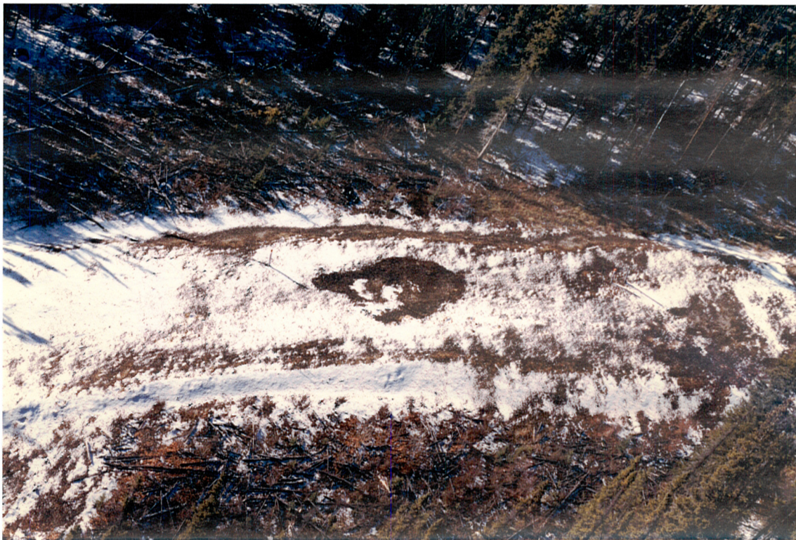
Plate 28. Slope 79, Whitesand North, KmP 279.0, Oct. 6, 1993. Aerial view of hot spot in the wood chip layer.
