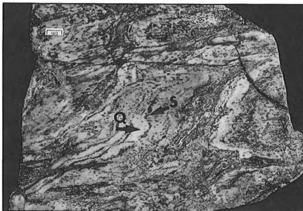
Figure 9. Transposed, quartz-veined (Q), and sulphidized (S) siliceous iron-formation, Wesmeg area.
