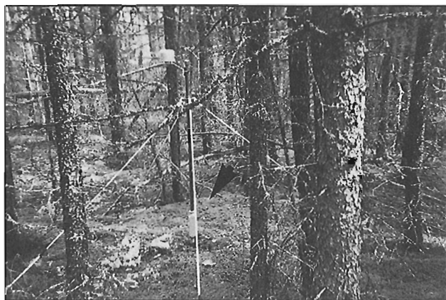
Figure 6. View of site 93 AG 3, Wrigley Hwy. km 504.7. Ground sensor is buried at arrow; remote sensor is on nearby cut line.
