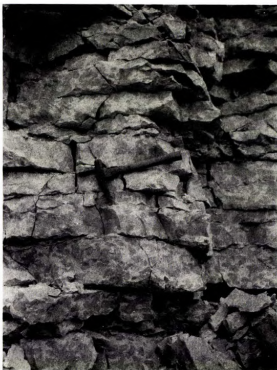
A. Thinly bedded, mottled Elm Point limestone in quarry of Canada Cement Company, Steep Rock, Man.
