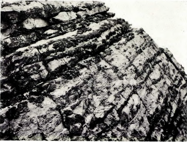
A. Bands and nodules of black chert parallel to bedding planes in Carboniferous high-calcium limestone, Exshaw, Alta.
