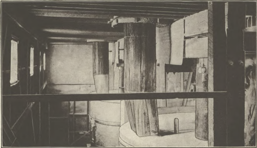
B. Back view of top of calcining kettles, showing stacks, Dominion Gypsum Co.'s mill, Winnipeg, Man.
