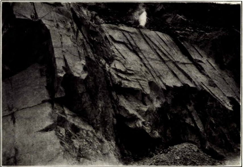
B. Quartzite quarry, Leitches Creek, Cape Breton county, N.S. Close-up view of the white quartzite showing the shattered condition of the stone.
