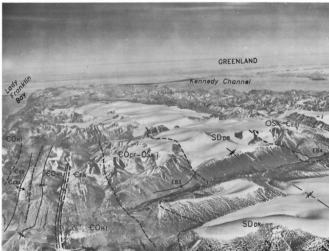
Frontispiece. Judge Daly Promontory, view to northeast. In the foreground is part of the key area shown in the geological map, Figure 1. Four major stratigraphic-structural belts are apparent, from left to right: 1) an area covered mainly by the carbonate member of the Hazen Formation ( CO_{H1} ) with outcrops of the Kane Basin ( CEK ) and Rawlings Bay ( C_{ERA} ) formations in the cores of two anticlines; 2) a belt of shelf carbonate and clastic units of Cambrian to Early Silurian age ( CO_{CF-OSA} : Cass Fjord to Allen Bay formations); 3) the Danish River Formation ( SD_{DR} ); and 4) another belt of shelf carbonate and clastic formations ( OSA-C_{ERI} : Allen Bay to Ritter Bay formations). The stratigraphy of the shelf succession on the northwestern limb of the Ninnis Glacier Syncline (section EB3) differs significantly from that on the southeastern limb (section EB4). (Part of oblique aerial photograph NAPL T-401-L-132.)
