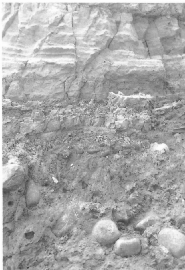
Figure 4. Poorly bedded diamicton of subfacies A2 sharply overlain by horizontal stratified sand of facies B. Cobbles in lower part of photo are about 15 cm in diameter (section 103). GSC 1993-209B
