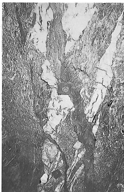
Figure 4. Quartz-carbonate vein cut by a narrow mafic dyke; note that the dyke itself is overprinted by the foliation. Steel plate in center of photo is 10 x 10 cm; Kierens deposit. GSC 1993-275B
