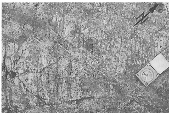
Figure 7. Closely spaced mineralized southeast-striking fractures cut by a barren east-northeast-striking fault. Compass is 7 cm wide. Location A in Figure 6. GSC 1993-220B
