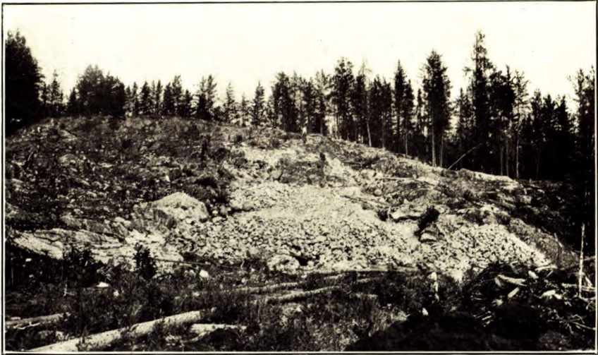
A. Outcrop of lithium-bearing pegmatite on property of Silver Leaf Mining Syndicate, Winnipeg river, Manitoba, looking east. Stock-piles of spodumene (left) and lepidolite (right) in foreground.
