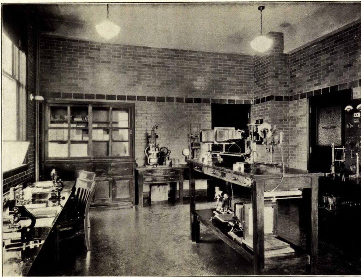
General view of the mineragraphic laboratory. The microscope table is shown at the left. The photomicrographic unit is shown in the centre foreground; the Harvard polishing machine and the mounting unit in the centre background; a portion of the spectrographic apparatus appears at the right.
