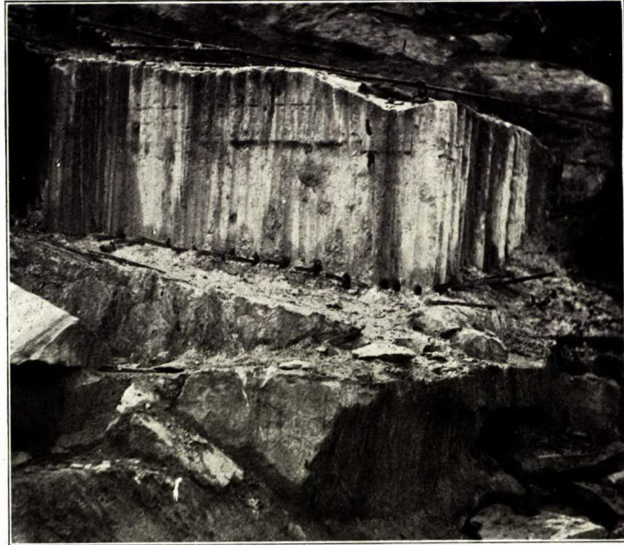
Raising a block of Marble by Shims and Wedges.
