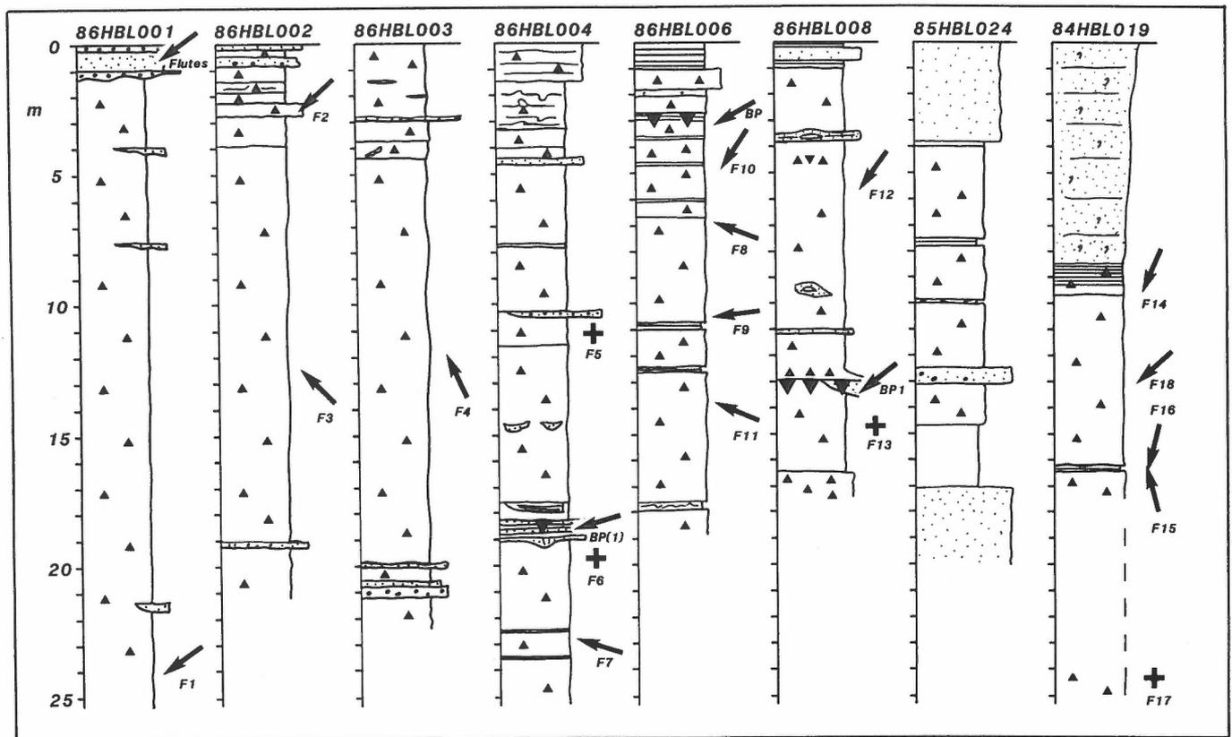
**Figure 16.** Severn River. Ice flow direction indicators. F numbers indicate fabric numbers from Figure 14. BP numbers indicate boulder pavement numbers from Figure 12. BP(1) indicates a striation measurement from one cobble. Arrows indicate ice flow orientation, with arrowheads arbitrarily directed to the south or west.
