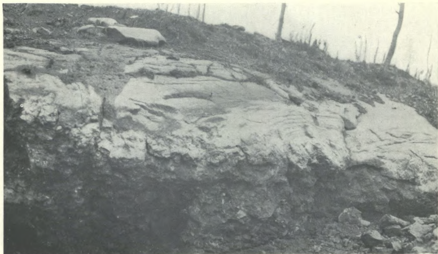
A. Part of vein from which ore shipment was made to the Mines Branch for test. The stripped surface is gneiss, with a thin band of pegmatite bordering the vein. (Photograph taken November, 1929).
