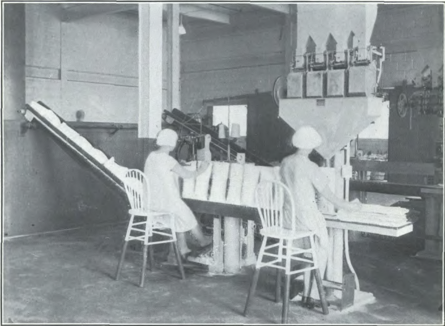
B. Automatic weighing, bagging, and sewing machines for table salt. Canadian Industries, Limited, Sandwich, Ontario.
