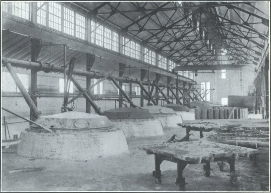
A. Fusion pots for caustic soda showing in right foreground the moulds in which the caustic solution is cast preparatory to shipment.
