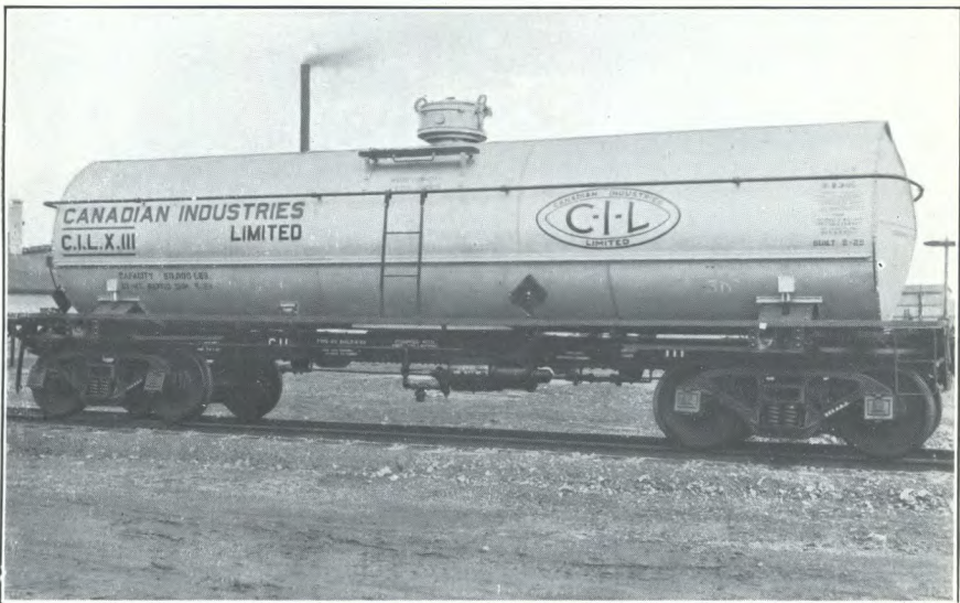
B. Tank car for the shipment of liquid chlorine. Canadian Industries, Limited, Sandwich, Ontario.
