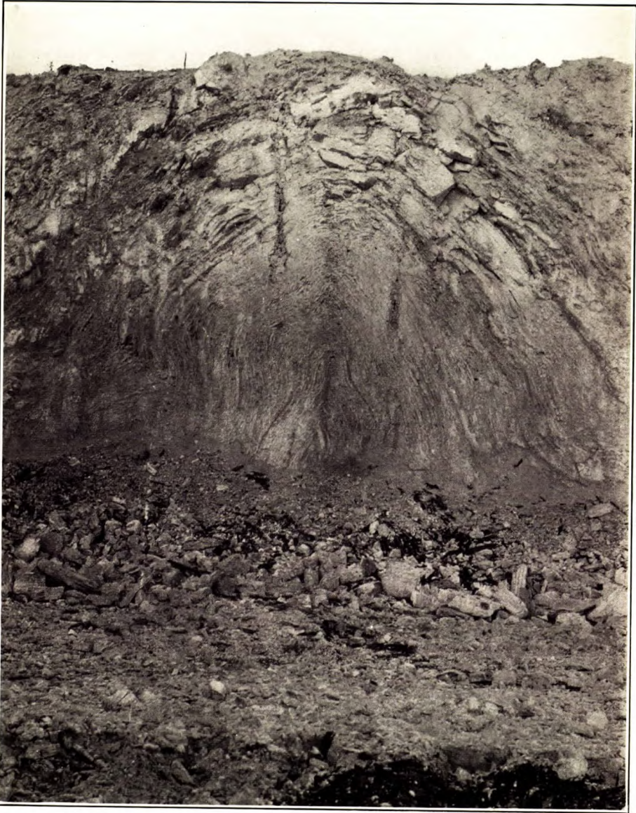
Face of quarry, Gypsum, Lime and Alabastine, Canada, Ltd., Gypsumville, Manitoba, showing anticlinal fracture of beds probably due to the alteration of anhydrite into gypsum.
