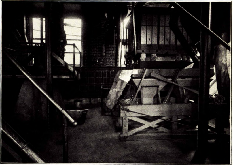
Ore dressing laboratory: Ferraris screen for coarse sizing in foreground; Keedy screen for fine sizing in background.
