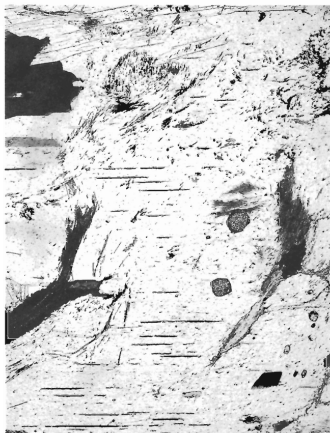
Figure 4. Photomicrograph showing sillimanite inclusions in large muscovites that crosscut the S_2 fabric. Long dimension of field of view is 3 mm.
