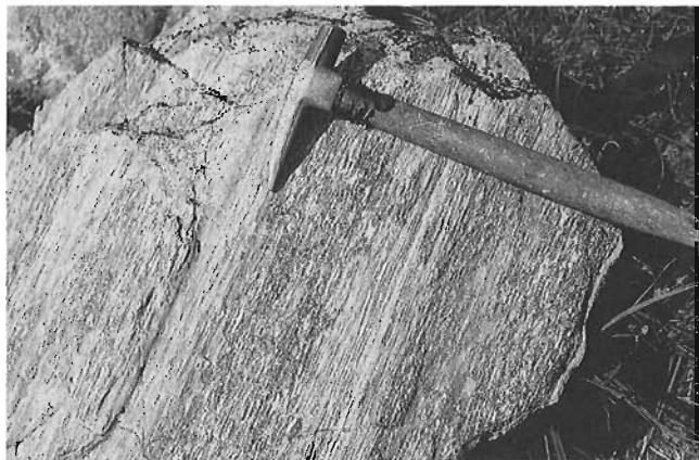
Figure 4. Strongly foliated quartz diorite in Thomas Lake shear zone, 1.5 km northwest of west end of Thomas Lake.
