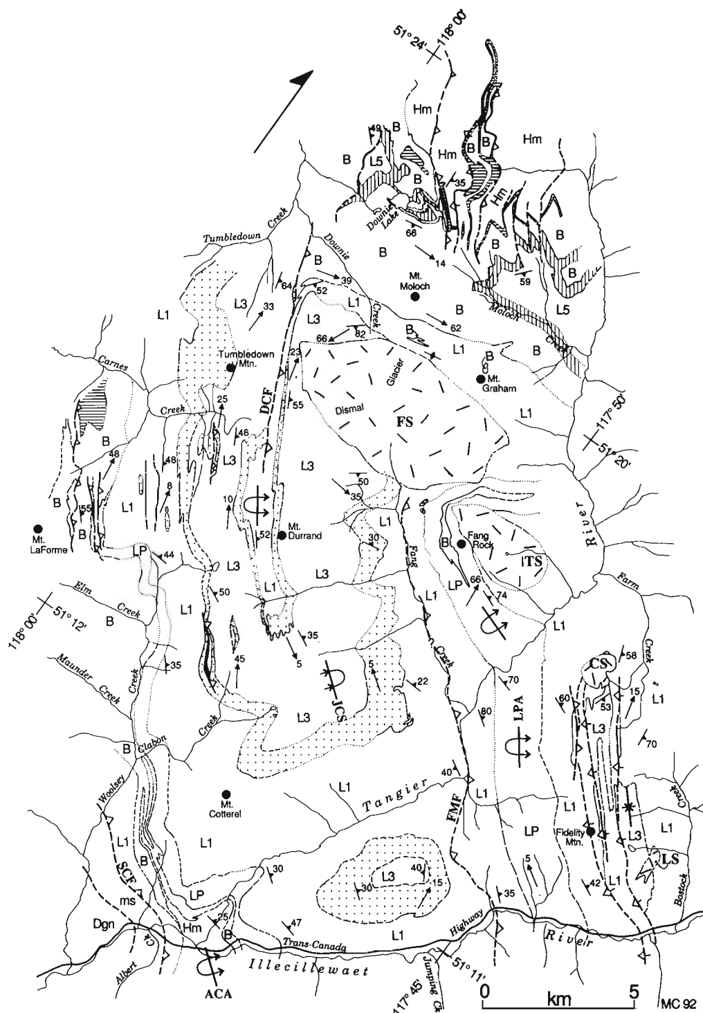
Figure 3. Simplified geological map of the Durrand/Dismal Glaciers area. Unit designators and patterns are as in Figure 2. Random dash pattern: Middle Jurassic granitic plutons. Structural data shown are strike and dip of dominant foliation and trend and plunge of dominant fold axes. Thrust faults have barbs on upthrown side; overturned thrust faults have ticks on lower plate. Other faults are steeply to moderately east-dipping. Geology to the north of Downie Lake is modified in part from unpublished mapping by R.L. Brown. Geology north of Mount Graham Lake is modified after Wheeler (1963), and that of the Albert Canyon anticline, after Zwanzig (1973). SCF: Standfast Creek fault; DCF: Downie Creek fault; FMF: Fortitude Mountain fault; ACA: Albert Canyon anticline; JCS: Jumping Creek syncline; LPA: Lanark Peak anticline; FS: Fang Stock; TS: Tangier Stock; CS: Corbin Stock; LS: Lanark Stock; Dgn: Devonian granodiorite gneiss (Clachnacudainn gneiss); ms: undivided metasedimentary rocks.
