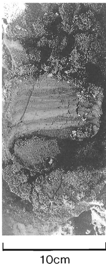
Figure 9. Photograph of split core from a site in central Lulu Island. Note interbedding of medium grained sands and laminated sands and silts. Between 11 and 11.2 m. See Figure 1 for location.
