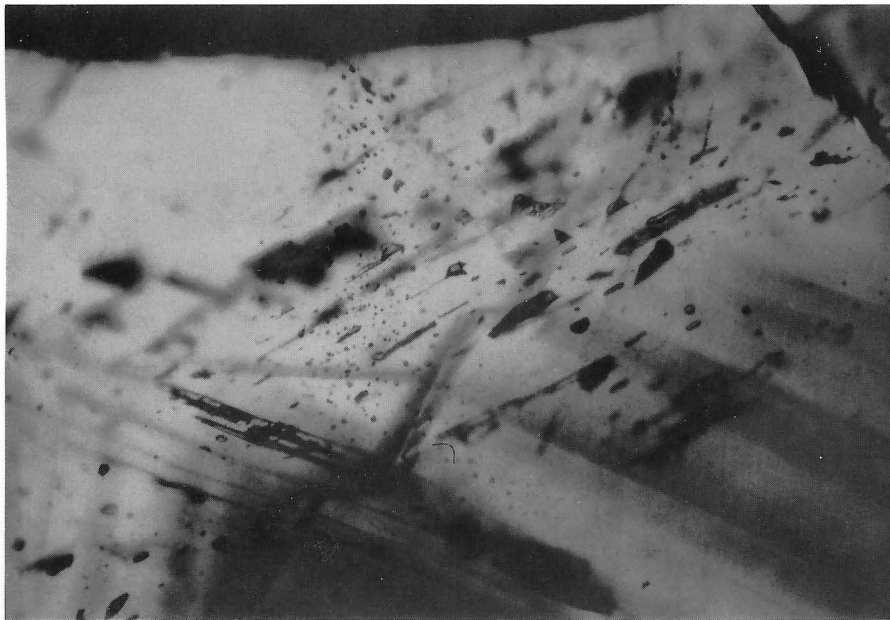
Figure 46. Close-up of area in Figure 12 showing concentration of inclusions on cleavage planes in sphalerite. The inclusions are concentrated at the junction between black and yellow sphalerite, which suggests that they are primary. Photograph Point. Field of view 0.8 mm.
