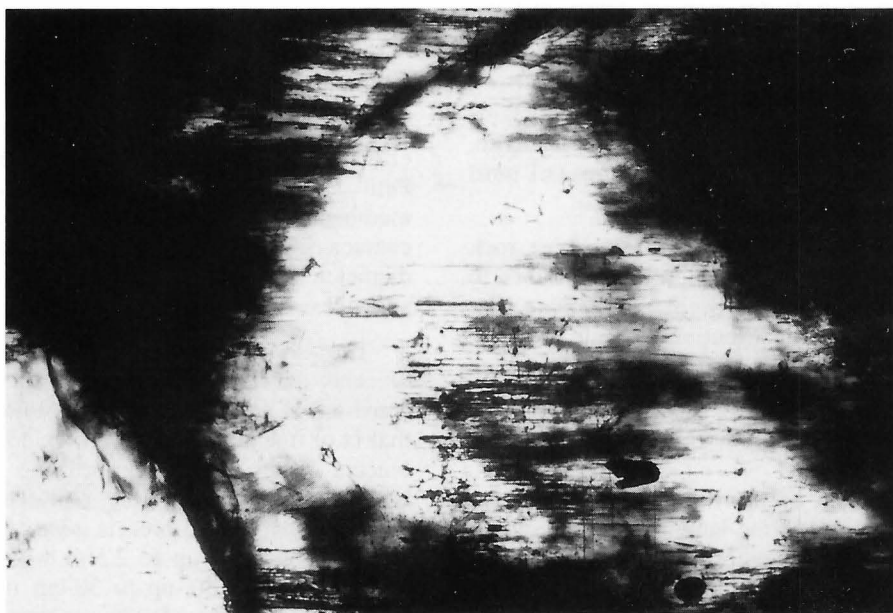
Figure 26. Photomicrograph of sphalerite that contains numerous marcasite inclusions. The marcasite is aligned along sphalerite cleavages and is so abundant that in places sphalerite appears black. Salmon River #3. Field of view about 1 mm.
