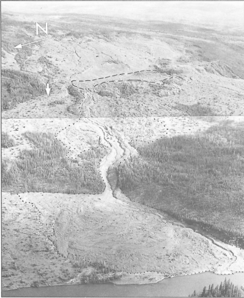
Figure 6. Low-level oblique photo of Surprise Rapids landslide taken in 1988 showing geomorphic element 6 (dotted line) and geomorphic element 7 (dashed line). Nested levee of element 4 indicated by small arrow. GSC 1991-114
