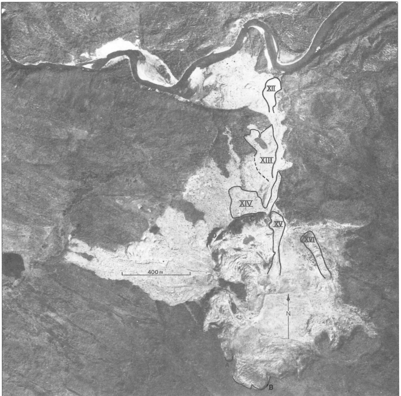
Figure 5. Enlargement of a 1968 airphoto of Surprise Rapids Landslide showing geomorphic elements, flows (Roman numerals), and flow source areas (capital letters), which are discussed in the text. NAPL A20695-100
