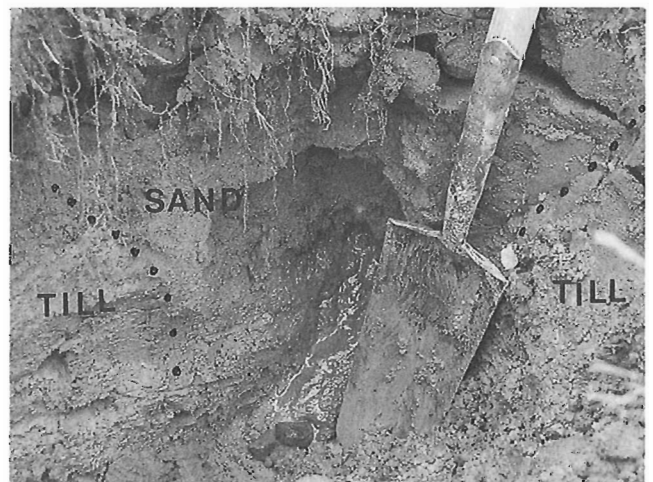
Figure 7. Sand wedge in till observed in a trench dug across a trough (GSC 1991-586 A).
