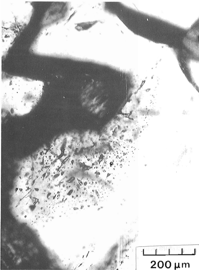
Figure 4a. Photomicrograph of cluster of primary fluid inclusions confined to growth zone defined by yellow sphalerite adjacent to inclusion-free white sphalerite.
