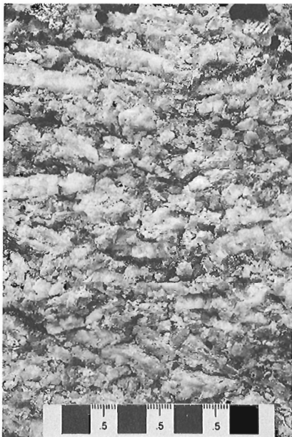
Figure 5b. K-feldspar-megacrystic biotite monzogranite distinguished within the Nova monzogranite (Fig. 2). Alignment of K-feldspar megacrysts is interpreted to be of magmatic origin. Scale is in centimetres. GSC 205300B.
