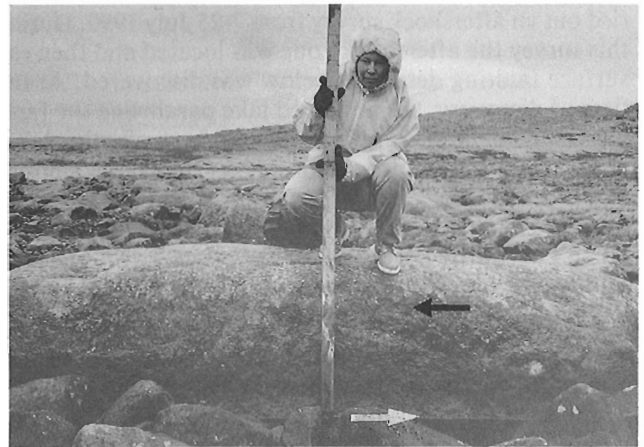
Figure 5. Shoreline uplift of 0.42 m on Lac Bécard near the southern end of the Lac Turquoise fault scarp. Pre-earthquake water level on this large boulder is indicated by black arrow, July 1990 water level by the white arrow.
