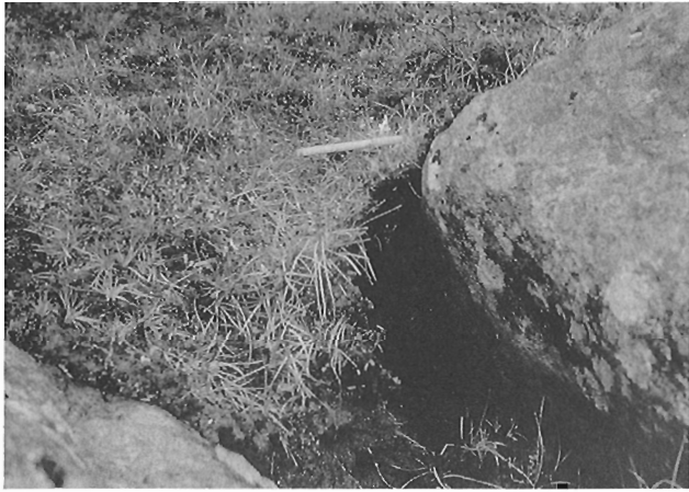
Figure 4. Fault offset of 110 mm between a boulder and formerly-adjacent peat along the left-lateral fault near the south end of the rupture.
