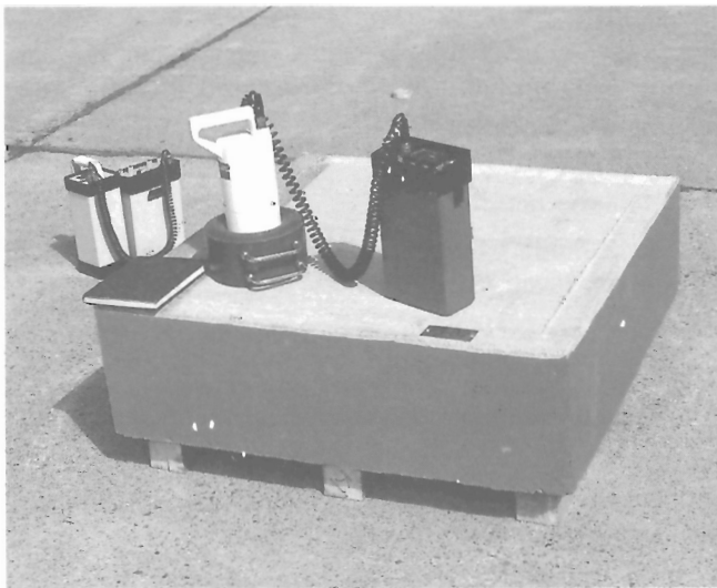
Figure 10. Homogeneity tests with lead-shielded spectrometer. GSC 1991-127
