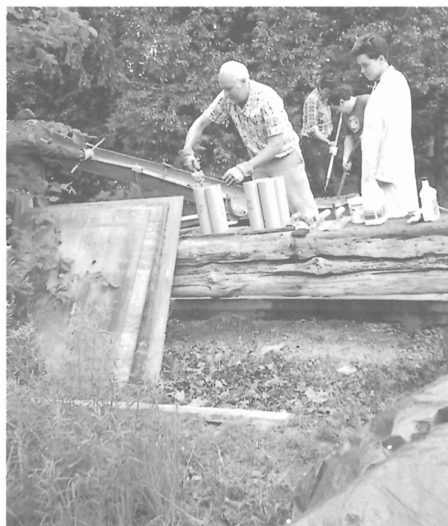
Figure 9. Concrete samples being taken for later analysis. GSC 1991-129
