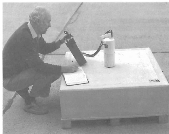
Figure 12. A portable spectrometer being calibrated. GSC 1991-126
