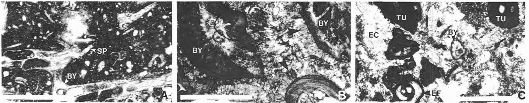
Figure 4. Microfacies of the Nansen(?) Formation in BP Graham C-52 well. A. Bryozoan (BY) silty wackestone with minor sponge spicules (SP); 2825 to 2850 m (9270-9350 ft.). B. Bryozoan (BY) grainstone cemented by radiaxial calcite (arrows); 2825 to 2850 m (9270-9350 ft.). C. Tubiphytes (TU), echinoderms (EC), bryozoan (BY) and encrusting foraminiferal (EF) silty packstone; 3030 m (9940 ft.). Scale bar is 1000 microns.
