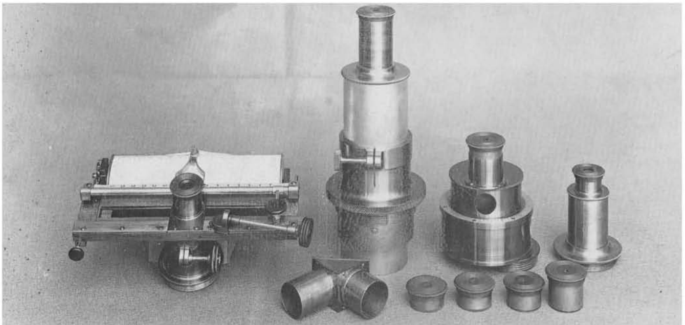
(Below) The eye-pieces and the position micrometer.
