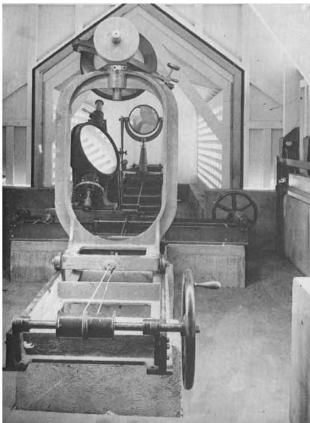
The mirror system of the coelostat. The large plane mirror in the left centre of the picture accurately follows the passage of the sun. It reflects the sun's image to the nearer, plane, mirror at the top of the picture, which reflects it to the third, most distant, mirror. This concave mirror focusses the image on the slit of the spectrograph, 80 feet distant.
