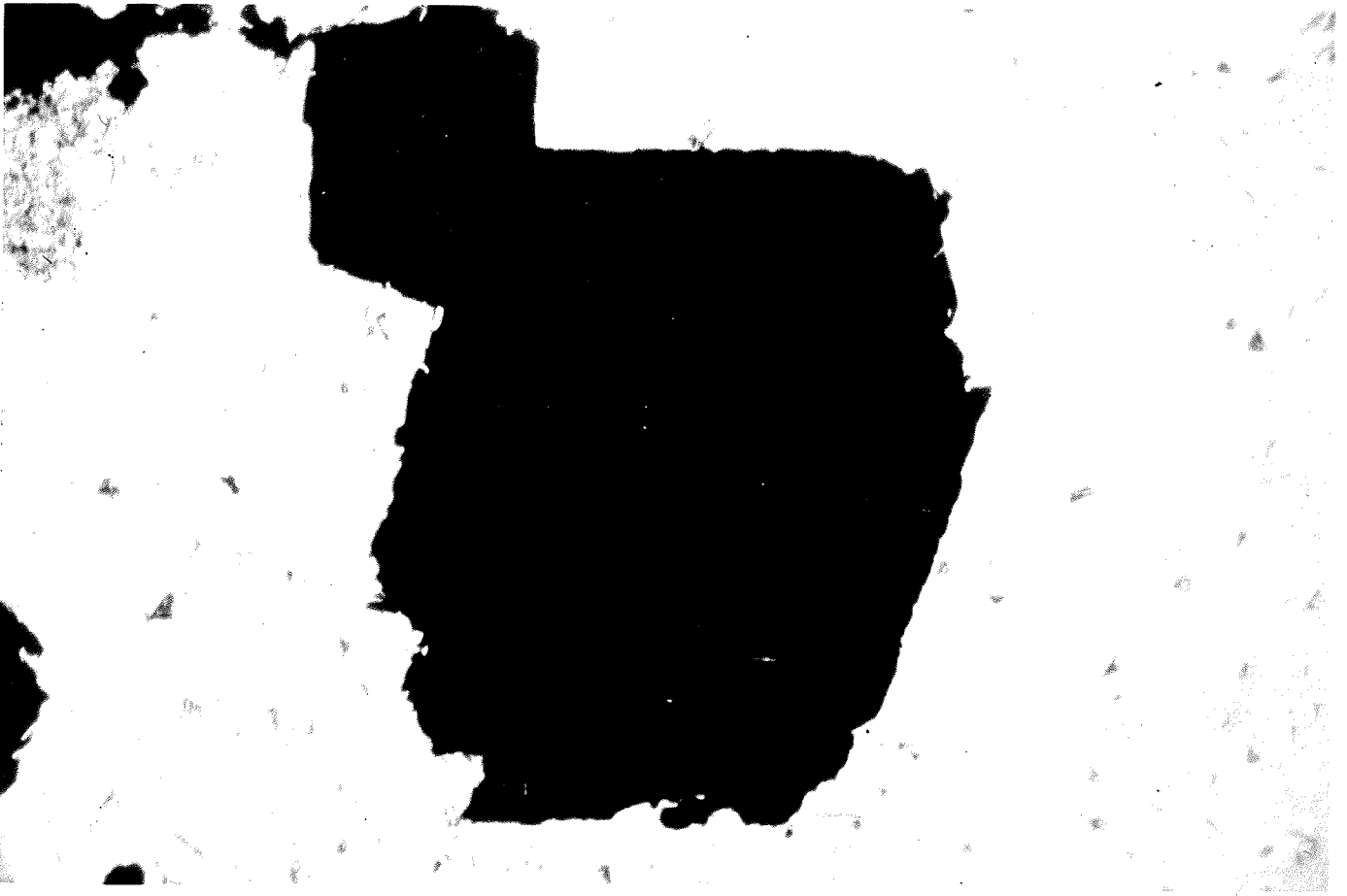
FIGURE 25 : Slightly fractured chromite with an iron -enriched halo surrounding a homogeneous core (sample STER-6B, field of view is 3mm wide).
