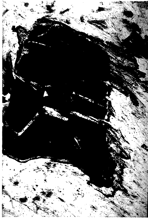
FIGURE 23 : Uvarovite growing within and around a fractured chromite grain (sample UVAROVITE, field of view is 3mm wide).
