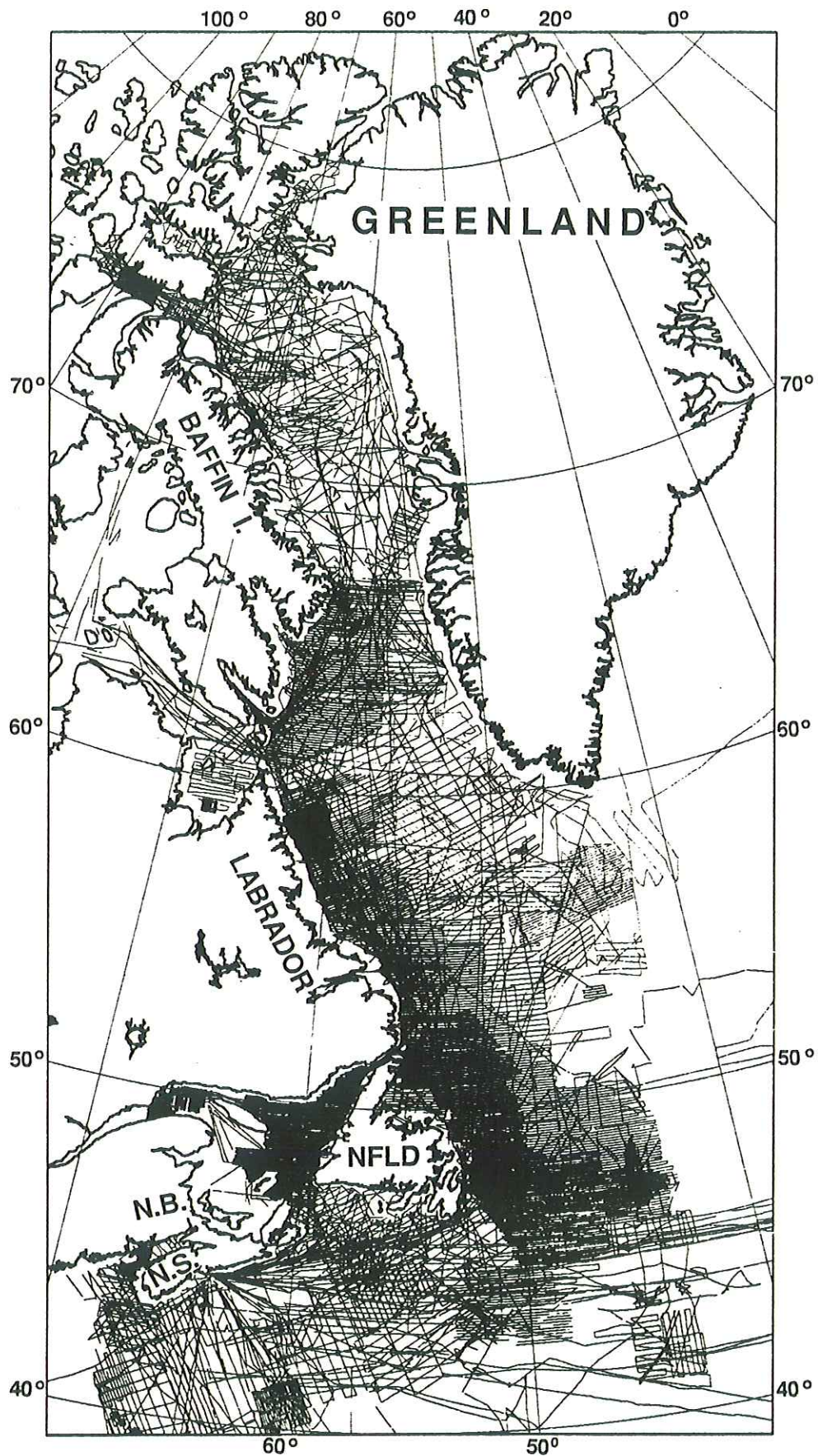
FIGURE 1. Ships' track chart showing where magnetic data were collected by AGC between 1963 and 1984.
