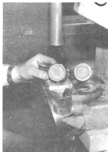
e. Cutting Coors ball mill gaskets with a 5 ton hand press.
