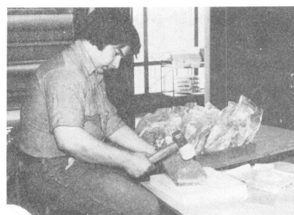
d. Hammering cemented stream sediment, lake sediment, etc., samples by a modified mallet in kraft paper bag placed inside a plastic bag.
