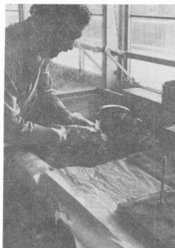
d. Washing Coors ball mill center parts. Note the use of a light gauge plastic bag as a glove.
