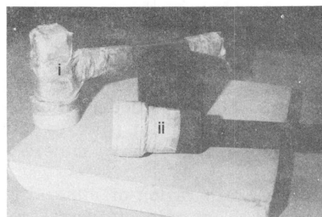
b. Ceramic sample preparation tools. Coors ball mill end caps taped to: i) mallet, ii) pestle, used for minimum contamination.
