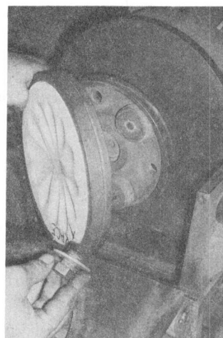
b. Braun pulverizer rotary disk-plate placed on rubber mounts to obtain a certain degree of flexibility for very fine grinding of samples.
