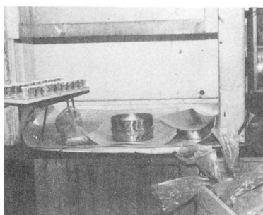
e. Set-up for sieving unconsolidated materials in a ventilation hood.
