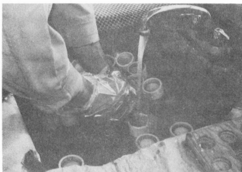
c. Washing Coors ball mill end caps with a stiff bristle circular brush.
