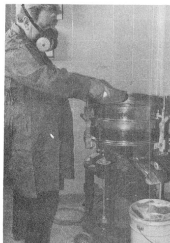
f. A 24 inch (60 cm) gyratory vibrating machine used to classify grains according to size. The screen frame can be dismantled for the employment of nylon, plastic, stainless steel, etc., screens. Ceramic balls together with a brush can be used to break up lumps in the sample and thus keep the screen free from clogging.
