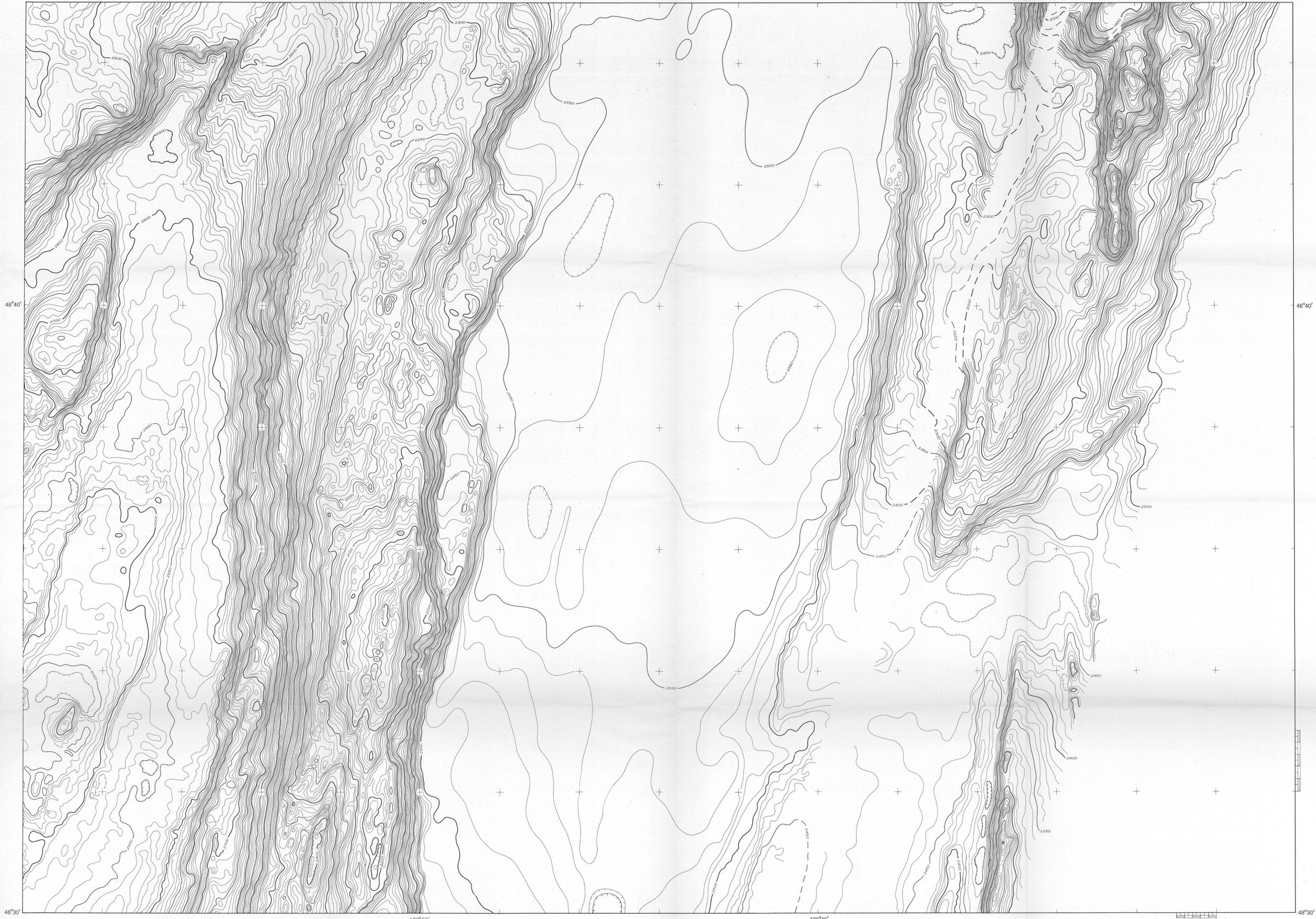
Depths are given in uncorrected metres assuming a sound velocity of 1500 m/s.
