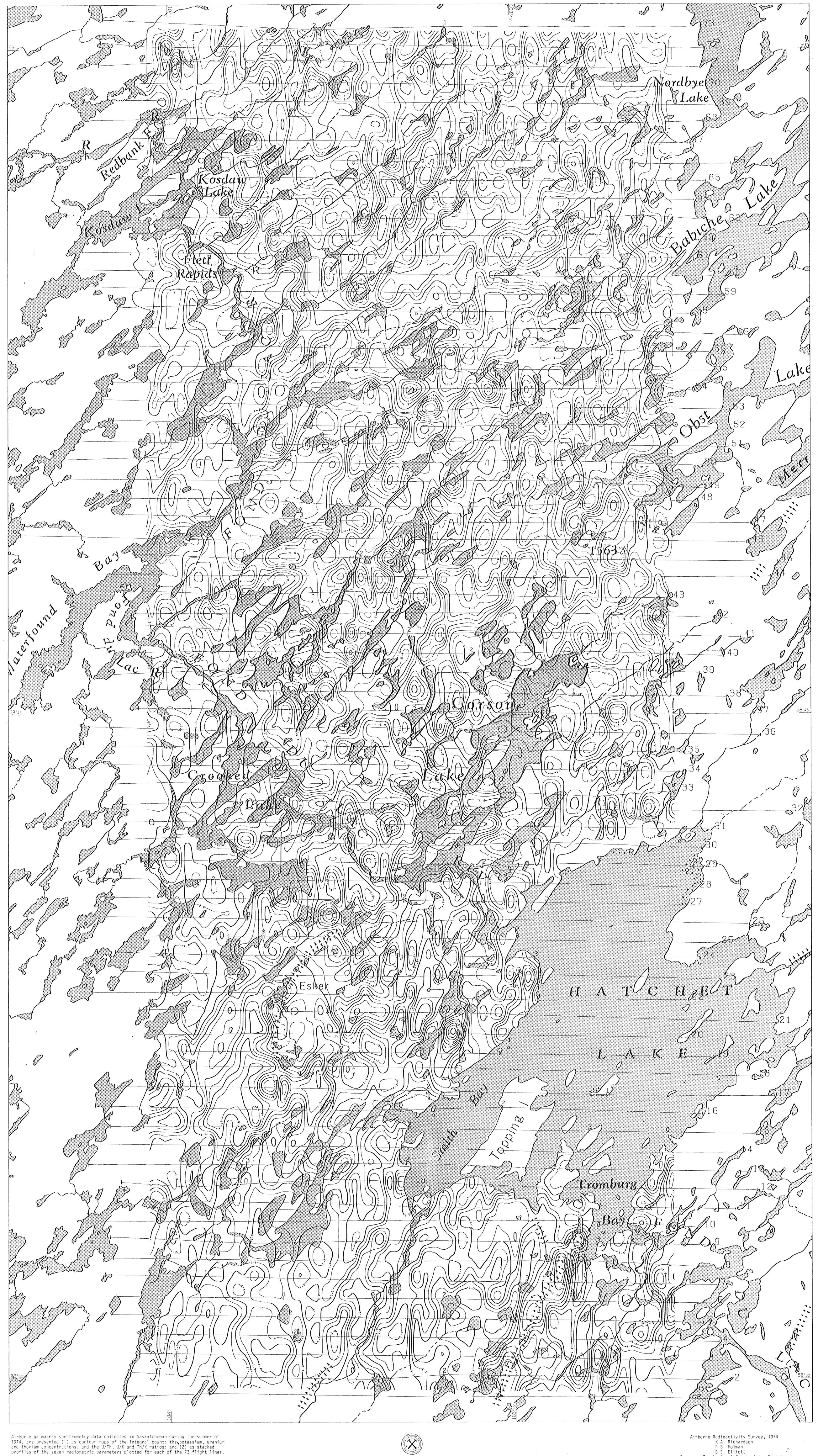
The airborne measurements were made using a four window spectrometer, with twelve 22.86 cm x 10.16 cm NaI(T1) detectors, flown at a mean terrain clearance of 120 metres and 190 km/hr. East-west flight lines were at 1/2 mile (approx. 0.8 km) line spacing, and the numbered flight lines are plotted on each of the contour maps.
