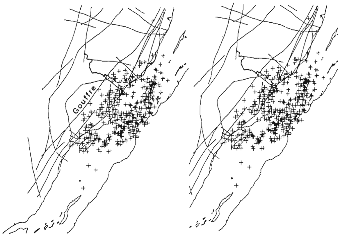
Figure 2. Stereo pair of overhead view of earthquakes in the Charlevoix Seismic Zone (similar to Anglin, (1984), but updated to include earthquakes until March 1989).
