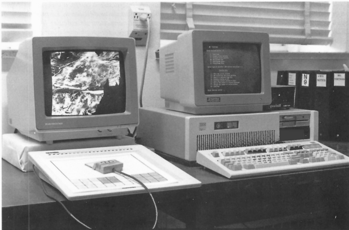
Figure 1. This photograph shows a complete workstation incorporating a IBM-PC/AT, 30 megabyte hard disc, 2 floppy discs, graphics tablet and monochrome and colour monitors. A grey-tone intensity image, generated from magnetic field data, is displayed on the colour monitor.
