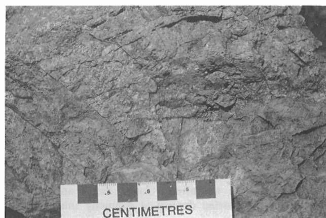
Figure 5. Fractured cataclasite in Jones Creek fault zone. Protolith is coarse Coryell syenite (compare with protolith in Fig. 6).
