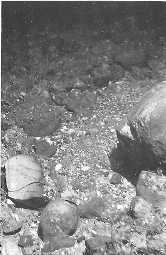
Figure 4.3 A bottom photograph of trench in the Strait of Belle Isle one year after it was cut. Notice the uncoloured area of the boulder which has been overturned by the plow. Base of photograph is approximately 1m.
