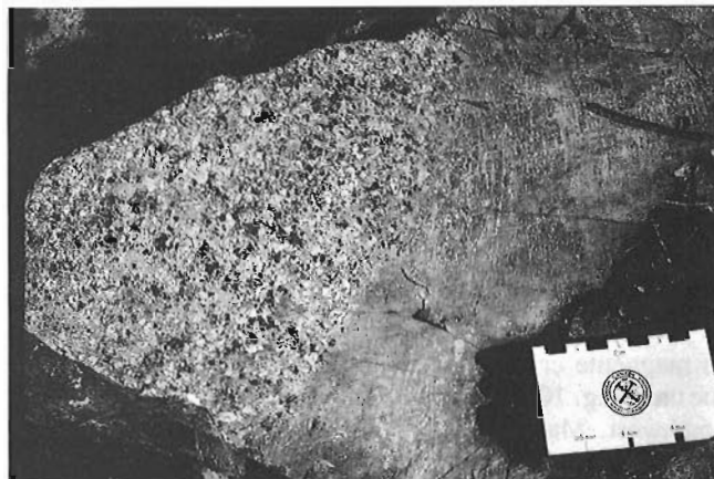
Figure 11. Contact of rhyolitic volcanic and quartz monzonite-granodiorite intrusion, sample site 267 (Fig. 2). GSC Photo 204718-A.
