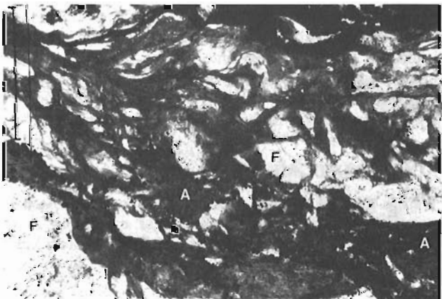
Figure 12. Fragmented feldspar (F) and fibrous reibeckitic amphibole (A) define a protoclastic texture, produced during minor shearing and alteration of alkali-feldspar syenite.
