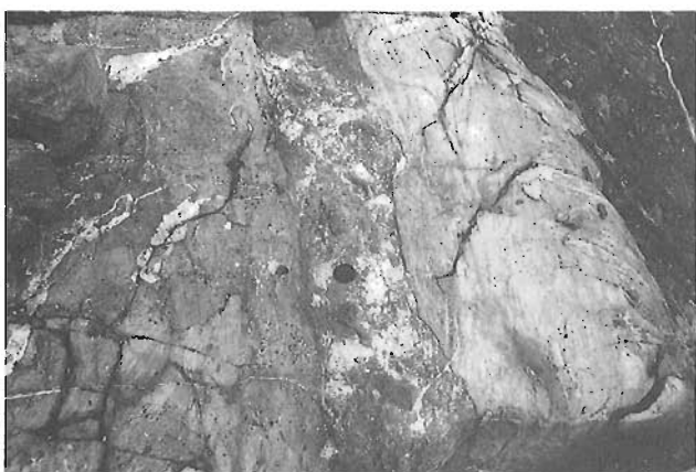
Figure 8e. Radioactive pyritic conglomerate bed in C member, Beaulieu Rapids formation, 63°04.47'N, 112°24.6'W. Lens cap providing scale is atop vertical drill-hole site of specimen 88RF52. Another hole 20 cm west with an inclination of 60°E (right) drilled through the conglomerate bed provided core specimens 53A, B, and C. Photo M. Stublely
