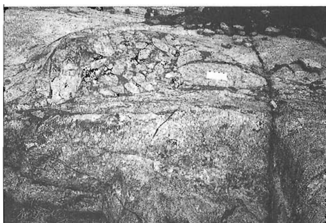
Figure 4. A breccia pod along a pseudotachylite vein. Plutonic rock fragments are included in black devitrified glass.
