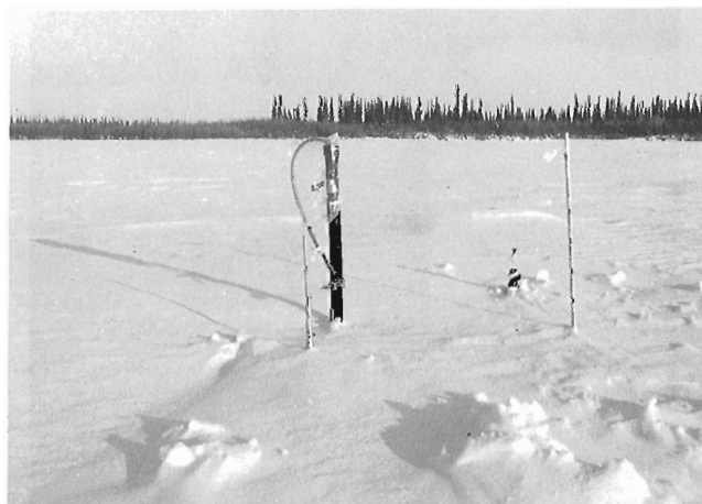
Figure 3. Site 1, Lake 1 on 16 March 1988. From left to right: heave tubes; thermistor cable; magnet access tube; snowstake.
