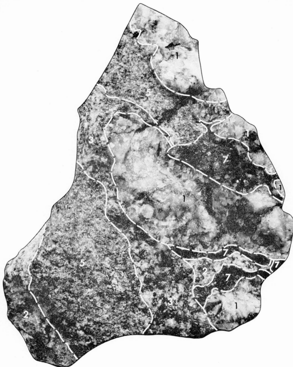
PLATE III. Opposite side of specimen shown on Plate II. A marked feature on both plates is the rapid variation in grain-size across a small distance. The mafic patch on the right-hand side consists of biotite and pyroxene crystals as much as an inch long. Numbers represent same facies as shown on Plate II.
