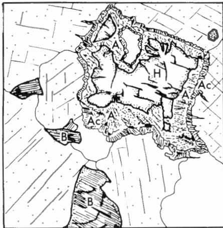
A. Hypersthene granodiorite (acid granulite) (56.48) showing the early stages of recrystallization. Hypersthene (H) is being replaced by anthophyllite (A) with an outer corona of actinolite (Ac). The red-brown biotite (B) is still relatively fresh (no recrystallization). Mag. X100.
