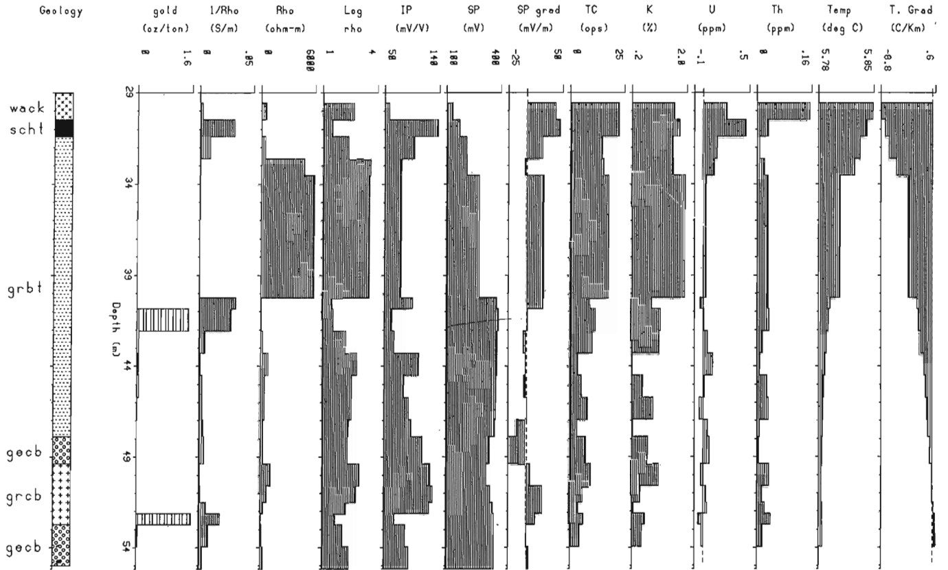
Figure 2.11. Correlations between the geophysical logs, gold assays and geological log for borehole 80-17. The geophysical logs are averaged over the gold assay sample intervals. The geology abbreviations are: wack - greywacke; scht - graphitic schist; grbt - grey flow breccia and tuff; geob - green carbonate; grcb - grey flow breccia.
