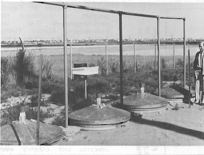
Figure 3.18. The two model boreholes located in Fredericton, New Brunswick at the Department of Mineral Resources. The 1.5 m thick 'ore zones' nominally contain 100 ppm U (BU-1-F) and 1000 ppm U (BU-2-F) for calibration of natural gamma ray logging tools. (GSC 203255-U.)
