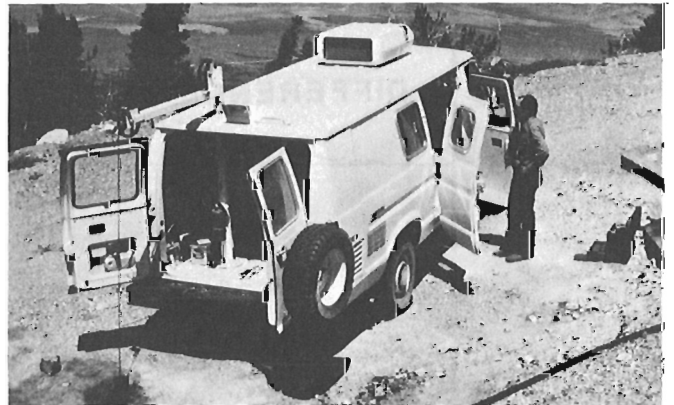
Figure 30.5. Logging a mineral hole near Ely, Nevada. The computer controlled data acquisition system is in the van. The draw work contains 3000 feet (about 1000 m) of cable. Electric power is supplied by a 5 kw gasoline power generator which is installed in the van.
