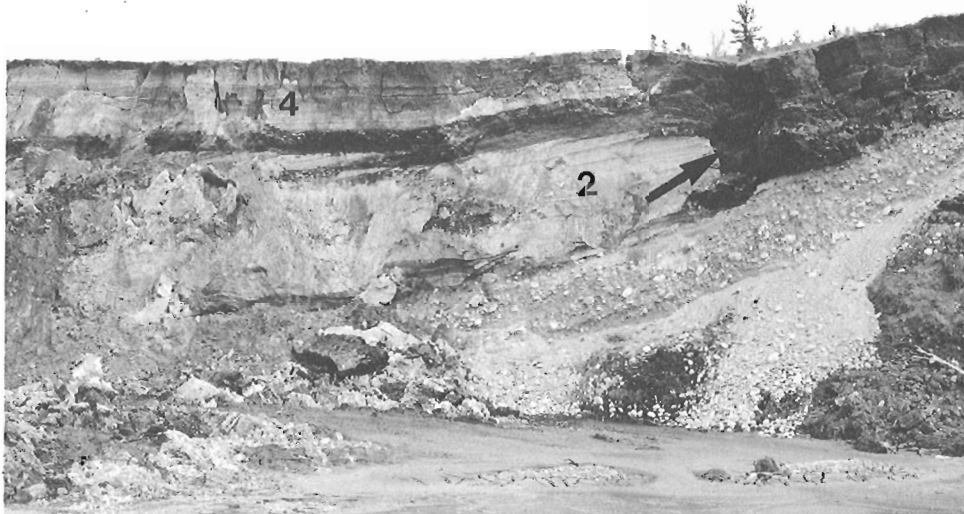
Figure 3. Photograph of the south end of the McNaughton Lake trench, May 1985. Numbered units are described in the text. Note the peat-filled channel cutting through units 1 and 2 (arrow). Compare with Figure 4.
