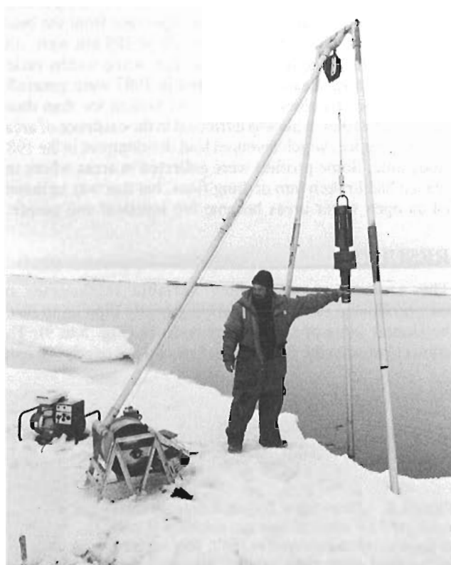
Figure 4. Photograph showing collection of a Benthos gravity core. The portable winch, powered by a Honda 3000 watt generator, is attached to the cantilevered tripod. Ice thicknesses at the lead edge were typically one to two metres.
