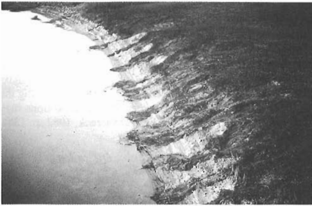
Figure 6. Debris flows extend across Mackenzie River beach at 30-50 m intervals for more than 50 km within fire limits.
