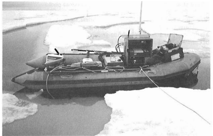
Figure 2. Five-metre Zodiac inflatable boat equipped for sparker seismic profiling in one of sixteen leads surveyed in 1987. The majority of the boat equipment was left attached during transfer between survey leads by helicopter, to prevent major disassembly of the system and navigation electronics.
