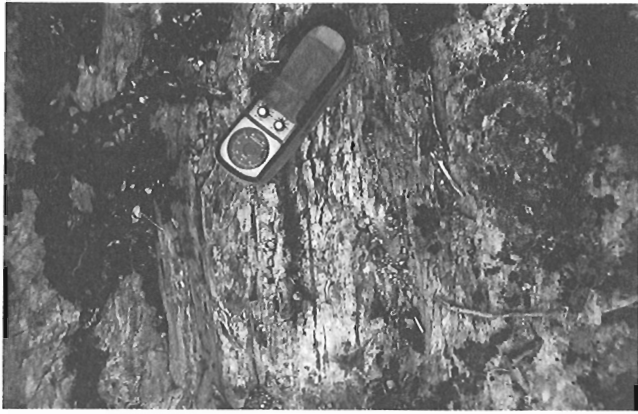
Figure 21. Mylonite with a single-radioactive lamella under centre of gauge on scintillometer.
