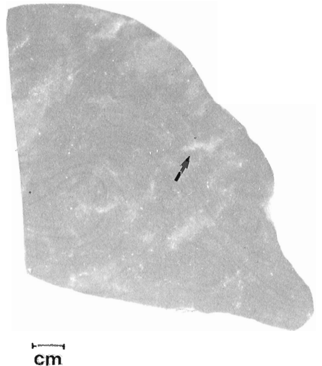
Figure 9. Autoradiograph (one week exposure) of a thoriferous phase (300 ppm) of the Quinnville carbonatite. Arrow points to wispy hematite rich radioactive area.
