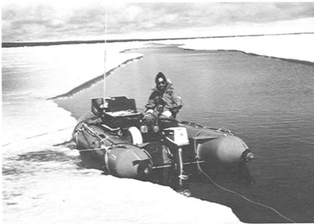
Figure 91.3. One of two five-metre Zodiac inflatable boats used during the 1986 program, shown in a lead equipped for sparker seismic reflection profiling.
