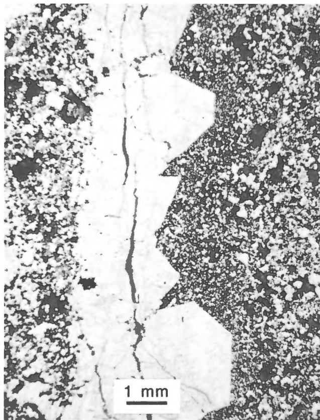
Figure 5. Photomicrograph (uncrossed nicols) of comb quartz layer in Granite II showing euhedral termination of quartz crystals approximately perpendicular to the layers; the very fine grained texture of the granite adjacent to the crystal faces probably resulted from pressure quenching related to the sudden release of the fluid phase in which the quartz crystals were growing. GSC 204152-T
