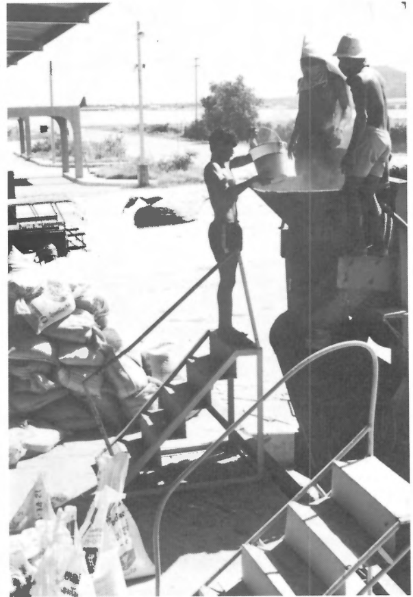
Figure 17. Loading the U-500 uranium concentrate into a cement truck.
