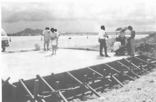
Figure 18. Checking the homogeneity of the pads with a portable gamma-ray spectrometer.
