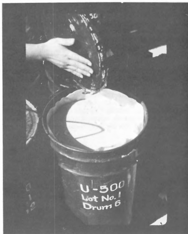
Figure 9. A drum of U-500 uranium concentrate prepared by mixing uranium ore with fine silica sand.
