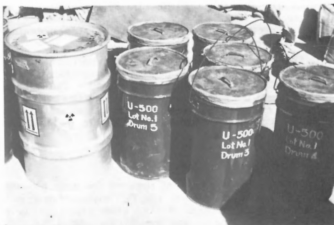
Figure 10. Drums of U-500 concentrate with the drum used to ship the Canadian uranium ore to Thailand.
