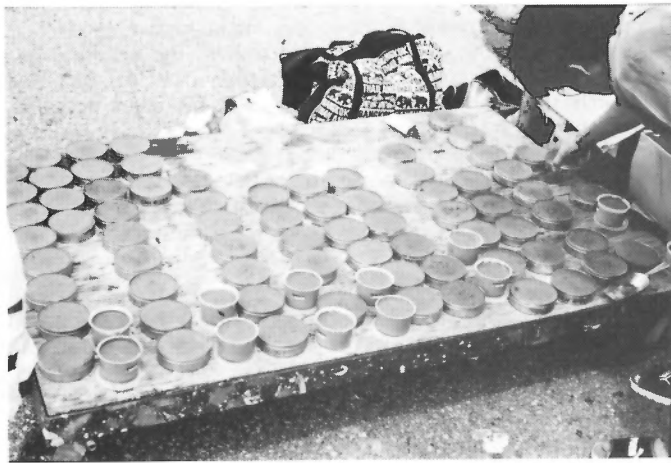
Figure 20. Metal sample cans for gamma-ray analyses and plastic containers for density and porosity.
