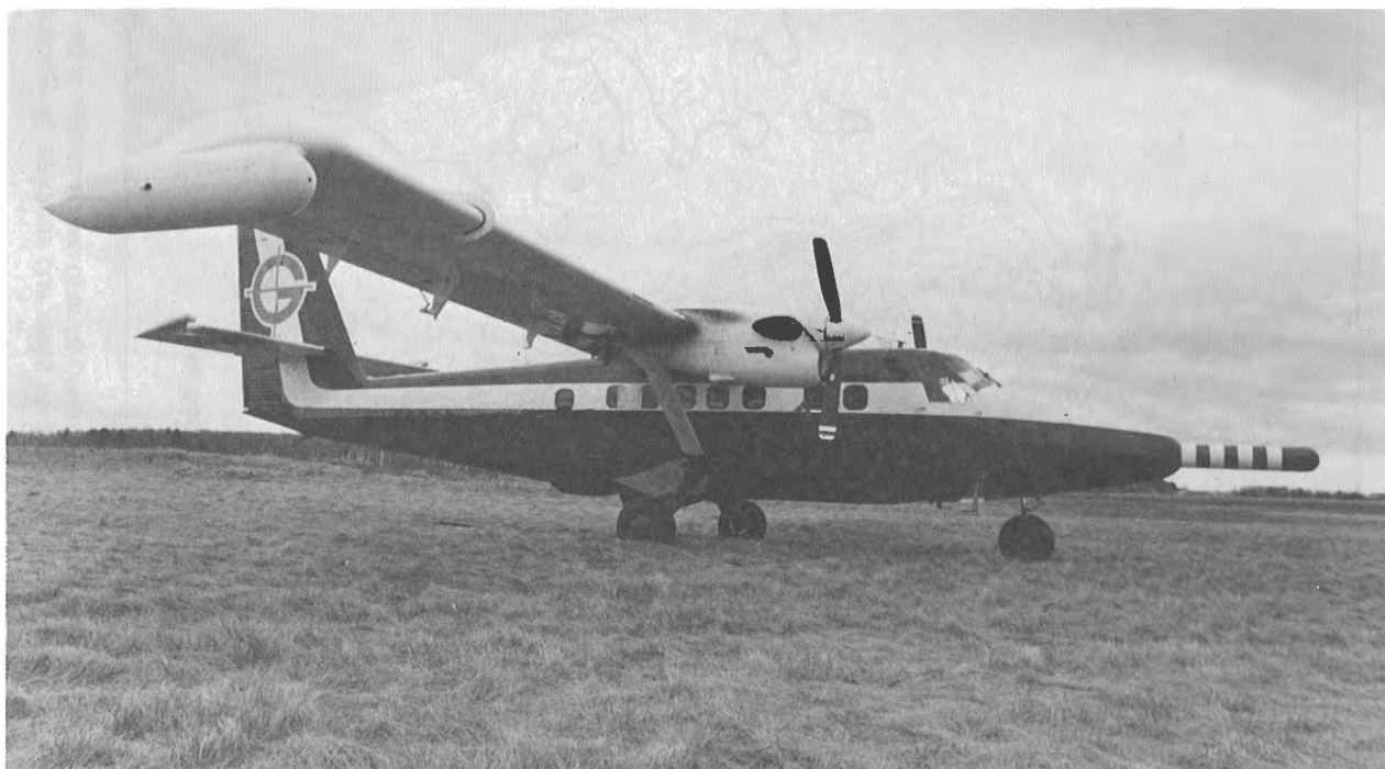
Figure 14.2. Geosurvey aircraft with Tridem coil pod at extreme end of the wing. Nose stinger contains the magnetometer sensor.
