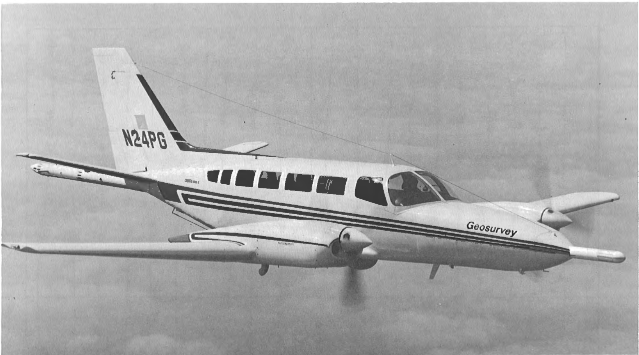
Figure 6.5. Nose-stinger installation of Totem-2A receivers (courtesy of Geosurveys International Ltd. of Nairobi).
