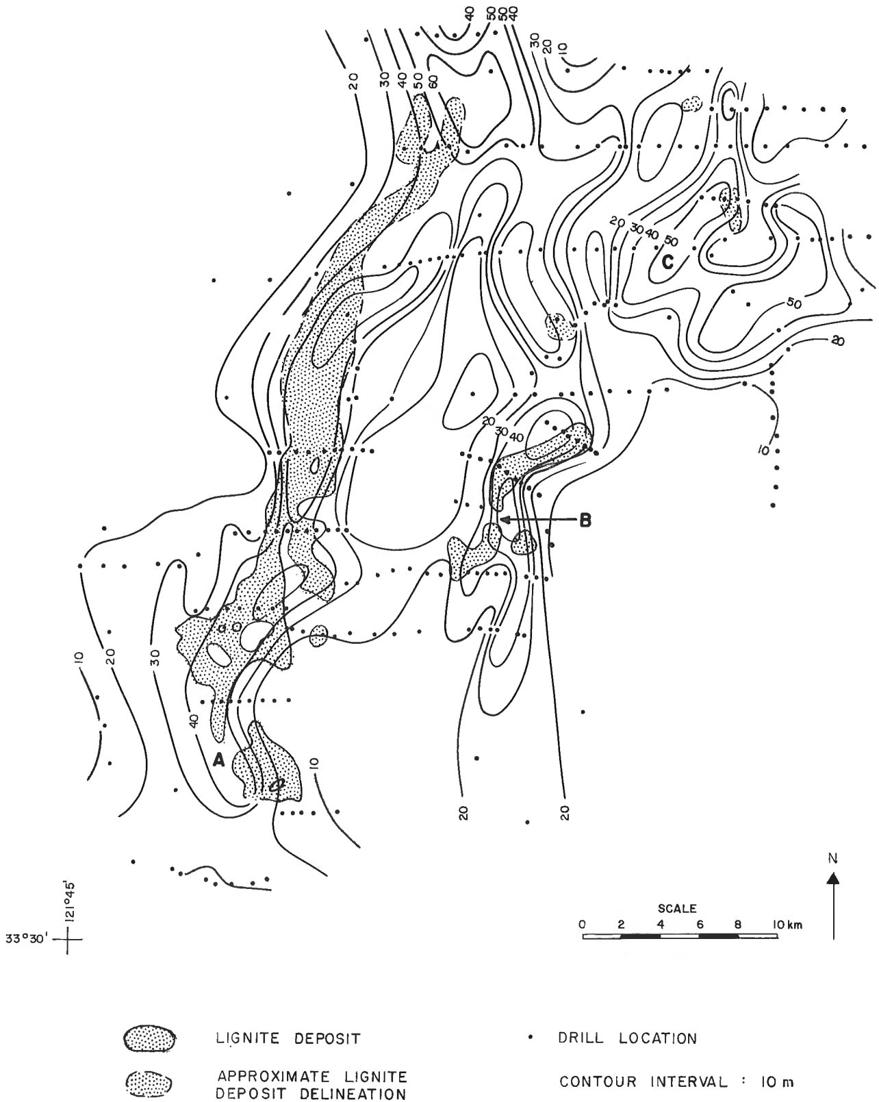
Figure 13.12. Drillhole depth to basement contours, Esperance, W.A. (after Whiting, 1983). The drillhole data give the depth to the weathered bedrock, whereas the AEM data indicate the depth to the fresh bedrock.
