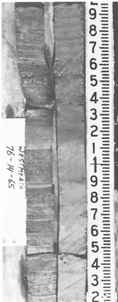
Figure 25. Sandy subfacies of Unit V from the western limit of the basin, showing cyclic alternation of thick sand strata grading upwards into thin red (dark bands) silty clay layers. GSC 203621-L
