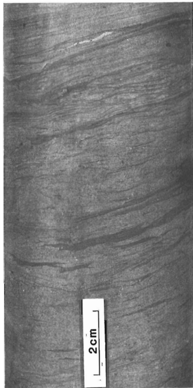
Figure 24. Dolomite marlstone, continuous to discontinuous kerogen laminae: (a) core, (b) photomicrograph (from Macauley and Ball, 1982).
